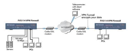
Figure 6-1: Secure access through FVS114 VPN firewalls
